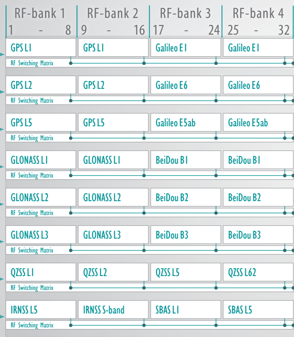
Example configuration of RFSIM modules with up to 32 RF-out signals
