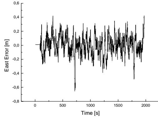
**Figure 4:** East error of filtered position
