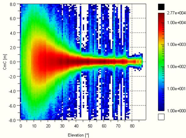
**Figure 20: Time differenced code-minus-carrier vs. Elevation (Station #15)**
