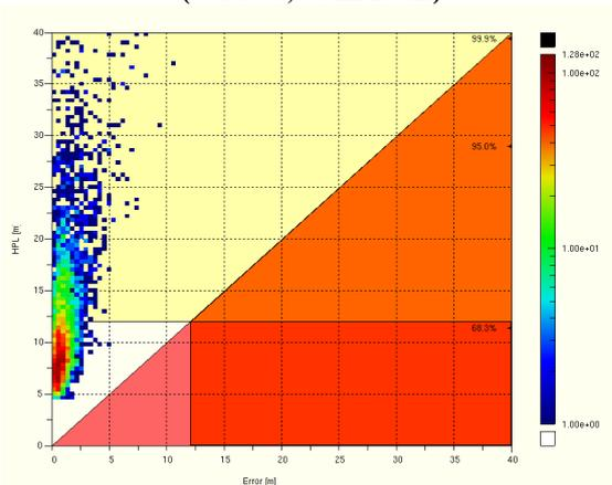
**Figure 9: GPS augmented: Stanford Plot (horizontal, HAL 12 m)**
