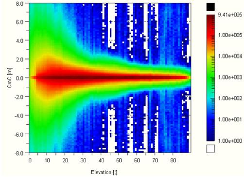
**Figure 16: Time differenced code-minus-carrier vs. Elevation (all Stations)**
