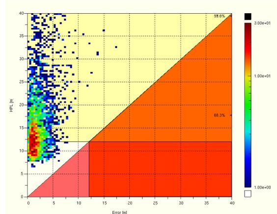
**Figure 5: GPS only: Stanford Plot (horizontal, HAL 12 m)**
