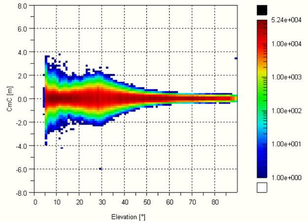
**Figure 21: Time differenced code-minus-carrier vs. Elevation (Station #19)**
