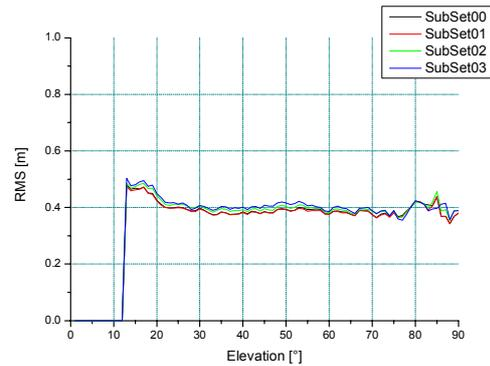
**Figure 28: Range Accuracy after Synchronization (RMS), all Station Sub-Sets**
