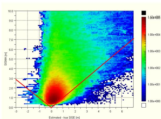
**Figure 38: Estimation error versus SISMA variable UERE budget**
