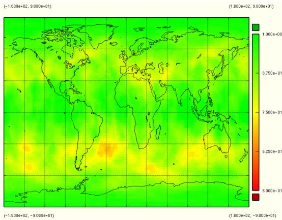
**Figure 7: GPS augmented: Availability (horizontal, HAL 12 m)**
