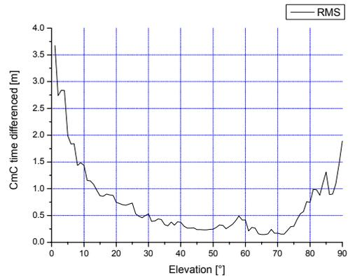
**Figure 17: Time differenced code-minus-carrier vs. Elevation (RMS)**
