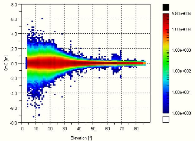
**Figure 23: Time differenced code-minus-carrier vs. Elevation (Station #24)**
