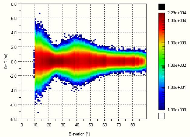
**Figure 22: Time differenced code-minus-carrier vs. Elevation (Station #21)**
