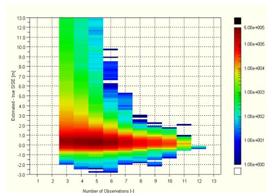
**Figure 34: Estimation Error versus Number of observations for satellites flagged as use**
