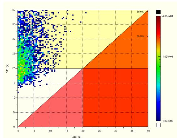
**Figure 6: GPS only: Stanford Plot (vertical, VAL 20 m)**
