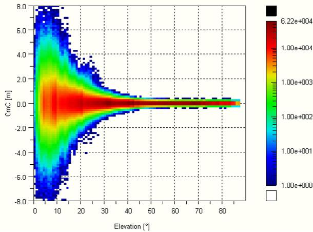
**Figure 19: Time differenced code-minus-carrier vs. Elevation (Station #08)**
