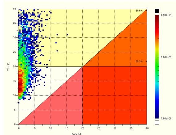
**Figure 10: GPS augmented: Stanford Plot (vertical, VAL 20 m)**
