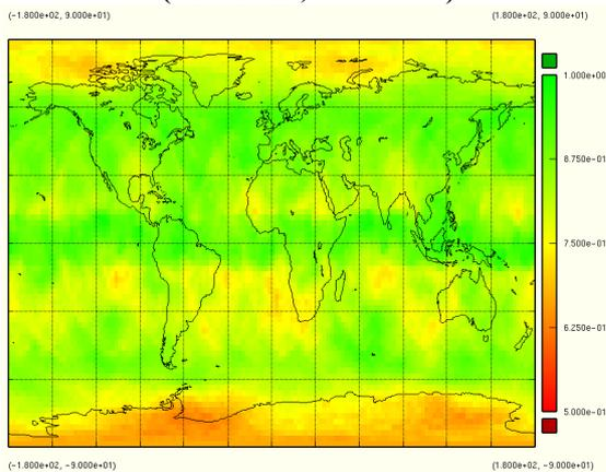
**Figure 8: GPS augmented: Availability (vertical, VAL 20 m)**
