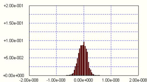
**Figure 25: Synchronization Error [sec] (T = 60 sec)**
