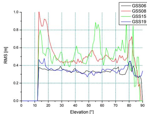
**Figure 29: Range Accuracy after Synchronization (RMS), selected Stations**
