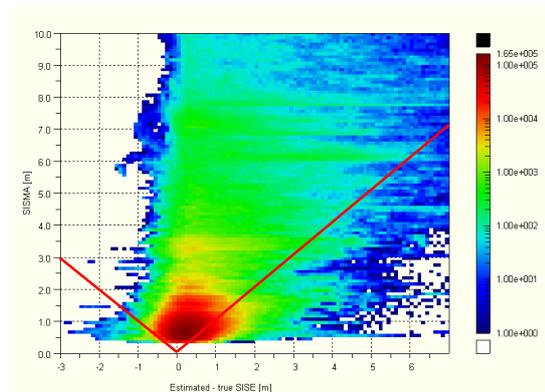
**Figure 37: Estimation error versus SISMA fixed UERE budget**
