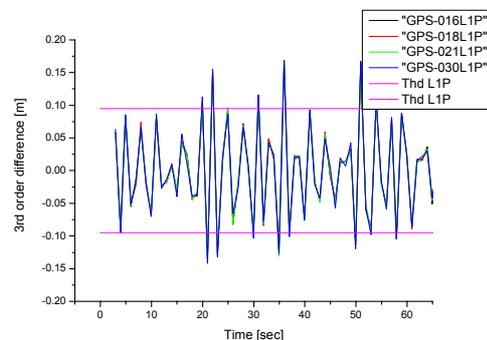
**Figure 14: 3<sup>rd</sup>-order time-difference on phase measurements to one station**
