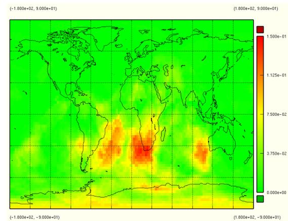
**Figure 11: GPS augmented: degradation of availability due to integrity monitoring (vertical, VAL 20 m)**
