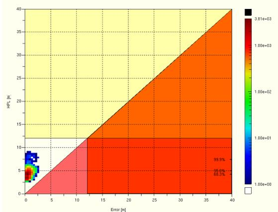
**Figure 12: Galileo Simulation: Stanford Plot (horizontal, HAL 12 m)**
