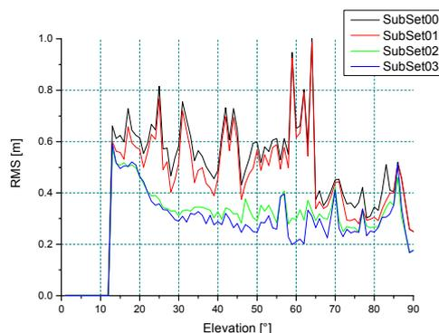
**Figure 24: Range Accuracy Before Synchronisation, all Station Sub-Sets**
